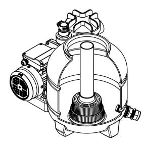
**4.** Insert the tube with the diffuser body inside the tank as above picture, then place the funnel on the tank's mouth and pour the quartz sand into the tank (about 20kg)
