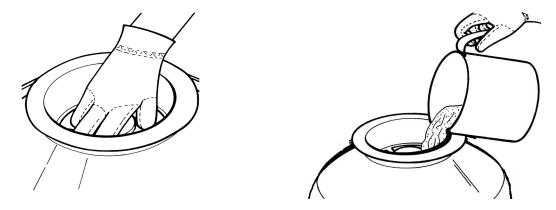
**5.** Take away the funnel, and then please make sure tank's neck is very clean. Put the O-ring on the valve and use clamp to fix the valve with tank. (the direction of "PUMP" port on valve needs to face pump out port).
