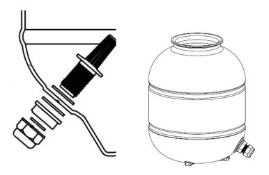
**3.** Press and turn the sand tank to mount it to sand filter support with correction direction (drain plug is at outside as below pictures).
