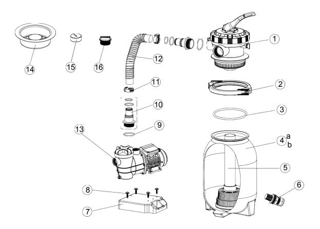
Parts Listing for 10" sand filter with pump
