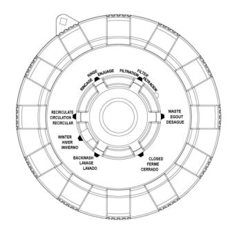
**RINSE** – After backwashing, with pump off, set valve to RINSE. Start pump and operate for about 1/2 to 1 minute.
