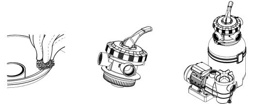
**6.**Connect the sand tank to pump with hose, hose clamps and hose adaptors.
