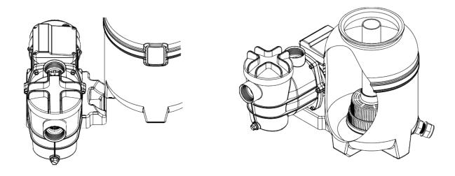
**4.** Insert the tube with the diffuser body inside the tank as above picture, then place the funnel on the tank's mouth and pour the quartz sand into the tank (about 13.6kg sands to fill into the tank)
